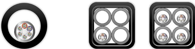
Figure 3. Comparison between traditional cabling in duct and micro cable, initial installation and full installation.
