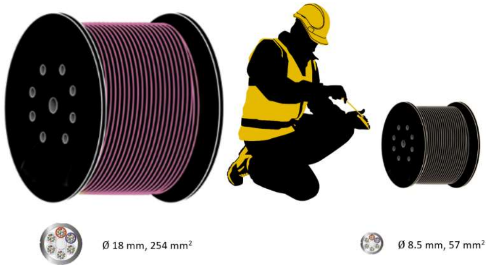
Figure 5. Comparison of standard duct cable and micro cable
